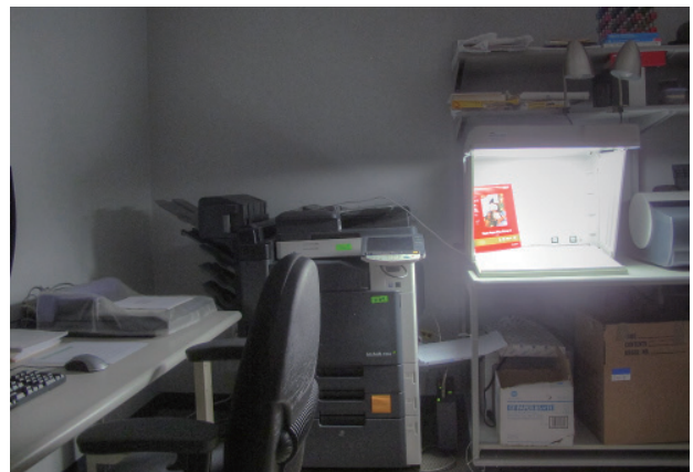
Fig. 8 Image created using three brackets with standard 2 stop difference (brackets 2, 4 and 6). Important details inside the light-box, such as the white square are lost using these brackets.
